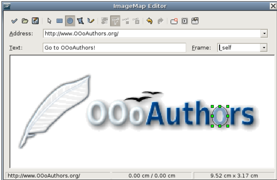
Figure 11: The dialog to create image maps. The last 'o' of the word Authors is set as an active hotspot
